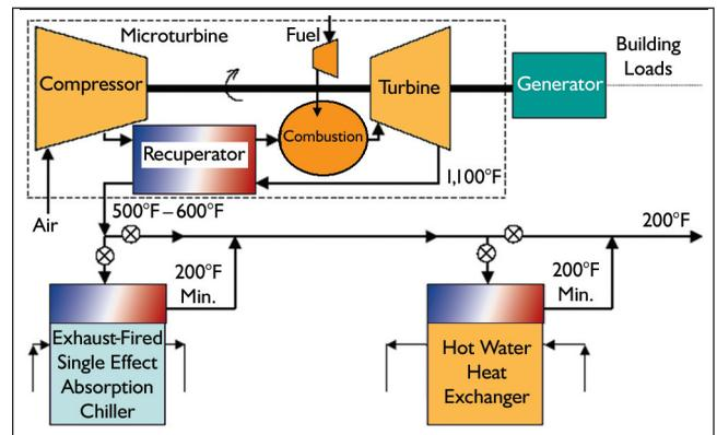
**Figure 1: A microturbine-based CHP system with single-effect absorption chiller cooling.<sup>1,6</sup>**
